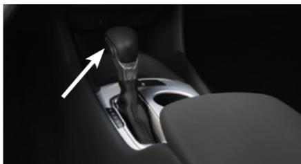
If vehicle speed is too high for the requested gear, the shift will not occur. Slow the vehicle to select a lower gear range.
